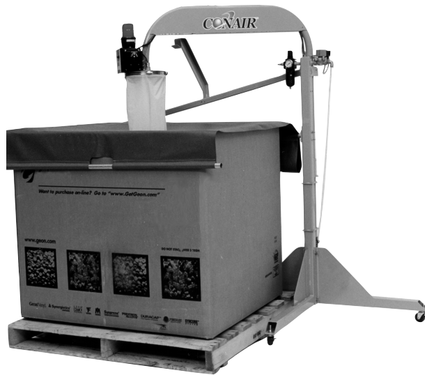
CAML-EVG shown with the optional retractable cover and one gaylord.
