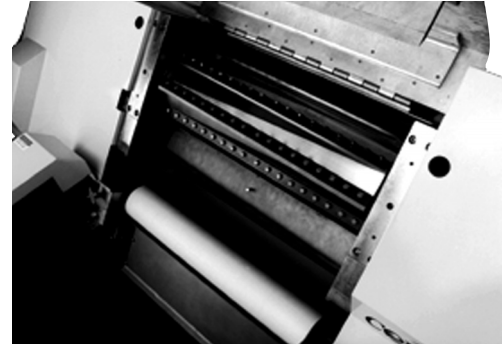
Cutting chamber with eight blade Pultrusion rotor. (Model 3032)
